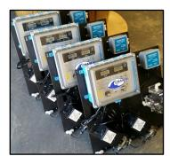
Our controller automatically maintains the chlorine residual and the pH level in your pool or spa. The controller's highly advanced sensors constantly monitor water conditions and activate the chemical feeds only when necessary, avoiding the over feeds common in manual feed systems and the resultant chemical waste and water imbalance. Our controller relieves you of
